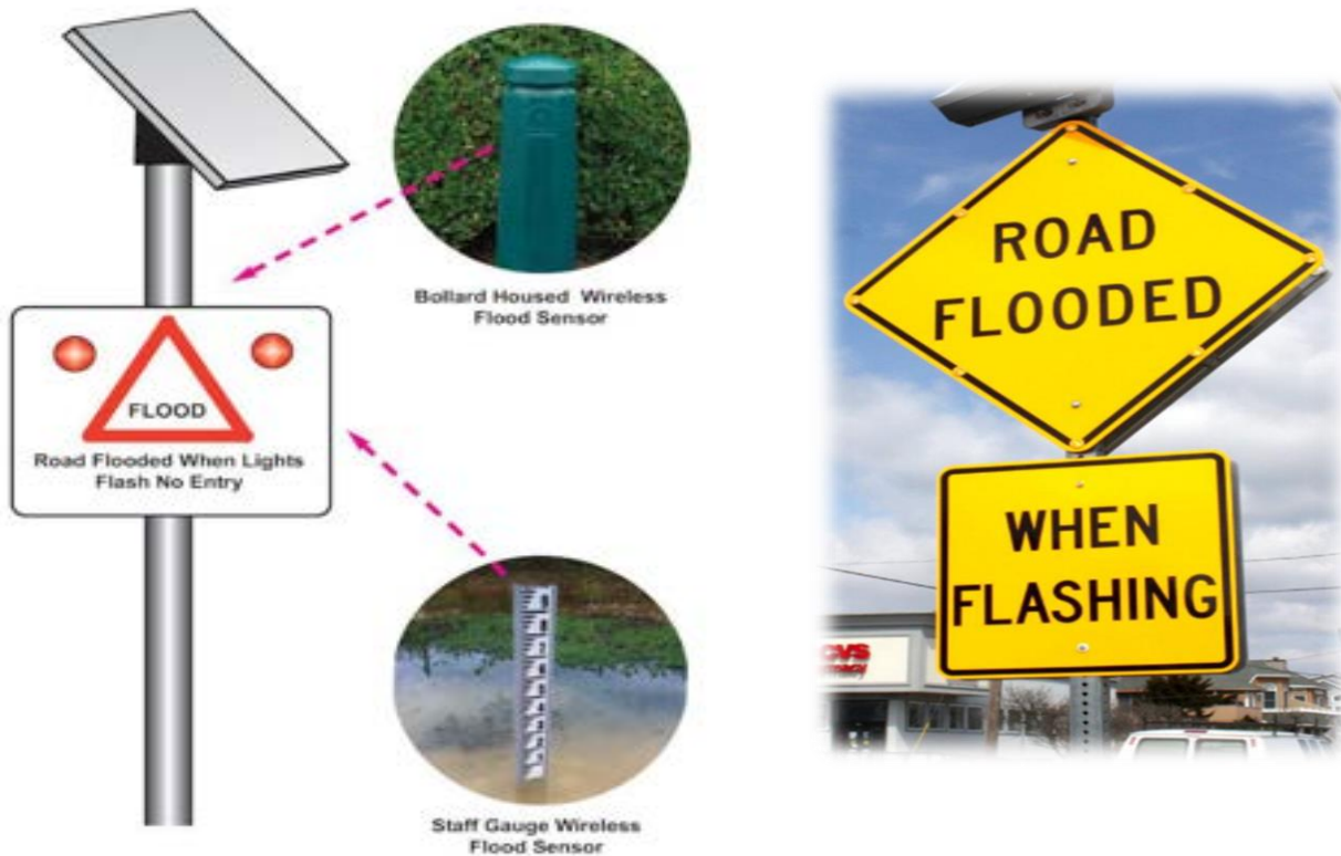
Figure 61: Automated flood warning sign with depth sensor gauge (Image Source: Radio Data Network, Cape May County Herald)
