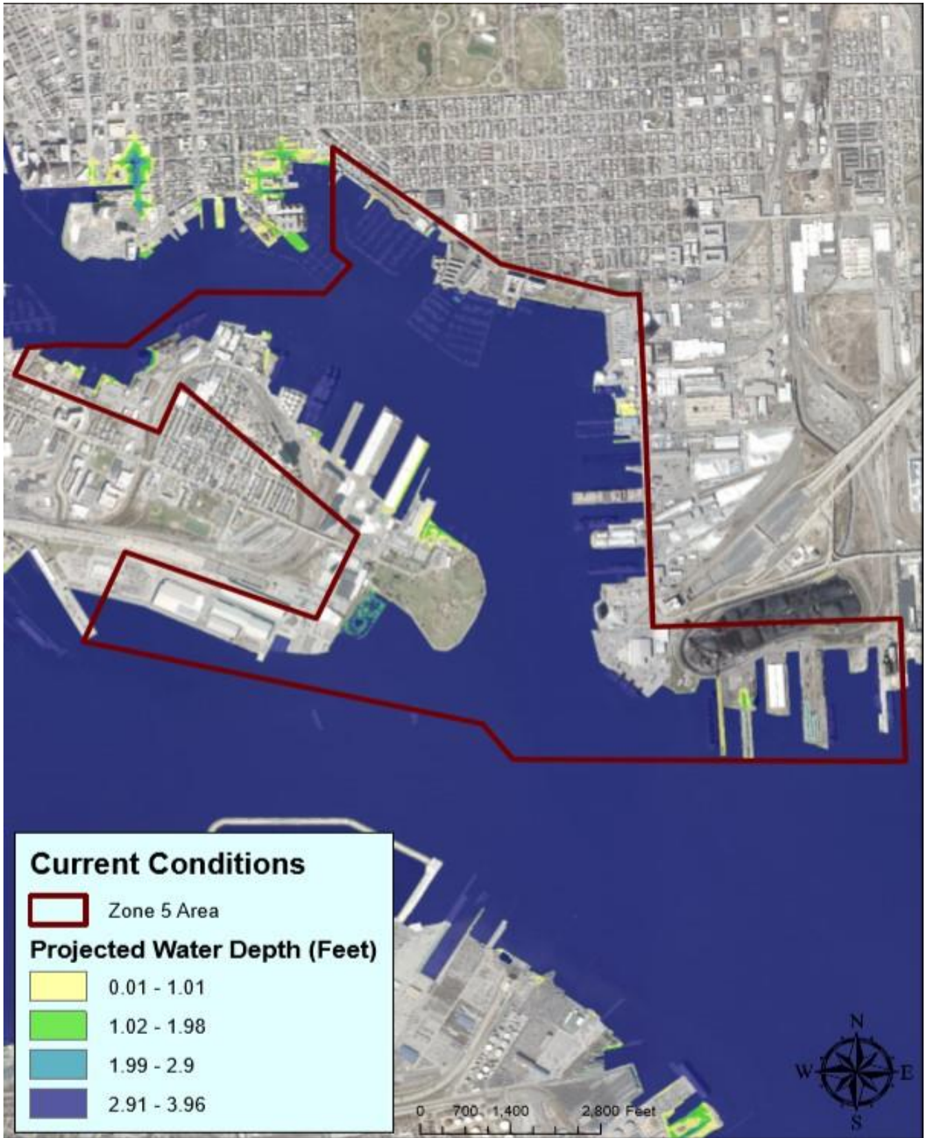
Figure 45: Zone 5 2015 baseline water depths (current conditions)
