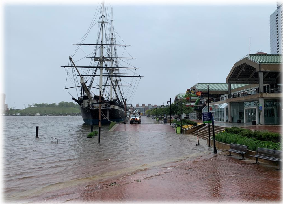
Figure 19: Nuisance flooding along the Inner Harbor promenade in May 2020. The northwest branch Patapsco River tidal gauge registered a 4.3 feet tide high during this period
