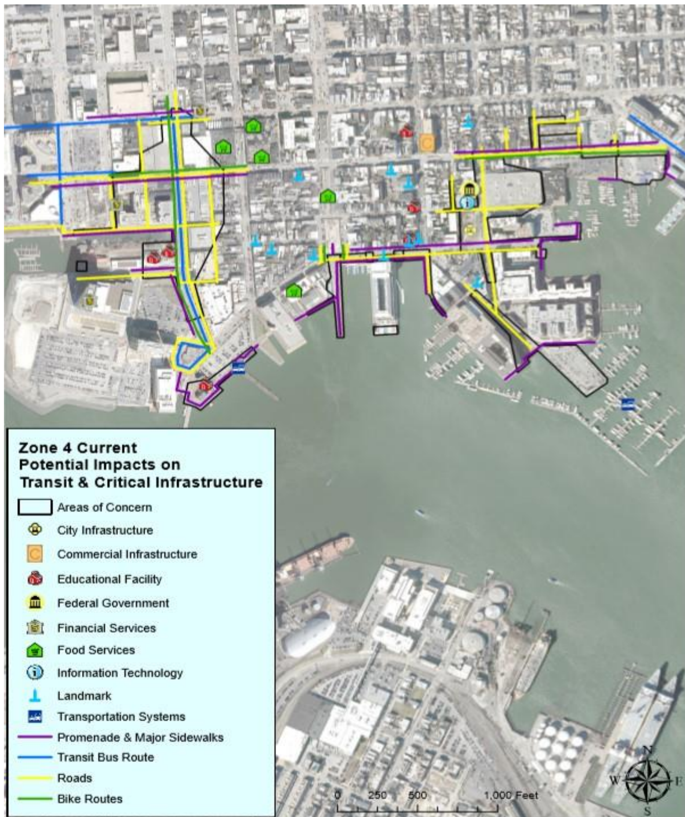
Figure 28: Zone 4 nuisance flooding effects on critical and city-owned infrastructure, along with affected transit routes based on current conditions
